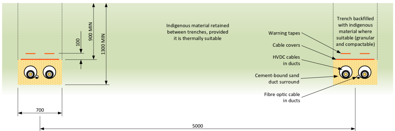
Plate 3.2 - Update of Plate 3.24 - Typical arrangement of HVDC and FOC cables in non-highway land (all measurements in mm)
